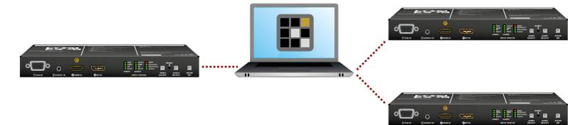
The transmitter (configuration) cloning of a UMX-TPS-TX100 series transmitter or wallplate is a simple method that eliminates the need to repeatedly configure certain devices to have identical (non-factory) settings. If the devices are installed in the same type of system multiple times then it is enough to set up only one device to fit the user's needs and then copy those settings to the others, thus saving time and resources.
