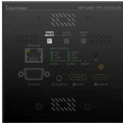
Desired video input can be selected by the **Video Select button** from the front panel. The selection order of the inputs depends on the model as follows:
