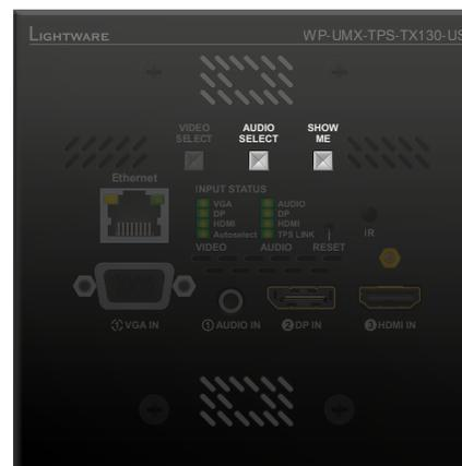
Press the **Audio Select** and **Show Me** buttons **together** (within 100 ms) to disable/enable front panel buttons; front panel LEDs blink 4 times when locking/unlocking. If the control lock is enabled and a button is pressed, front panel LEDs blink 3 times.
