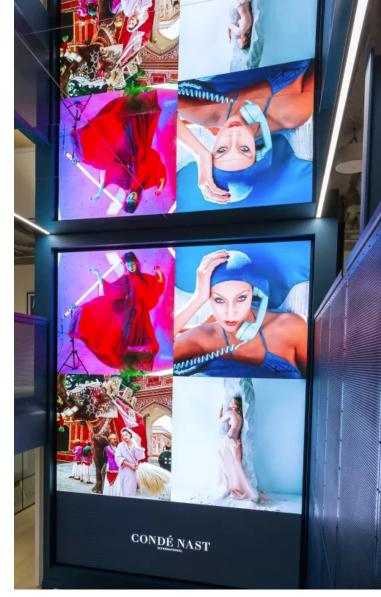
design in conjunction with primary contractors BW. The wall was ultimately based around Christie's Velvet Apex Series indoor LED tiles, which feature an ultra-fine 2.5mm pixel pitch, 16:9 aspect ratio, UHD resolution and advanced monitoring capabilities, while multiple Crestron systems provide control.
