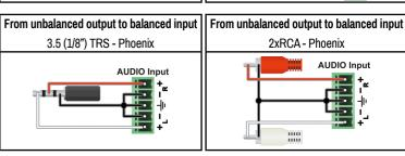
For more information about audio cable wiring see the user's manual of the device or the **Wiring Guide** on our website www.lightware.com/support/guides-and-white-papers.
