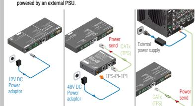
1 UMX-TPS-TX100 transmitters are PoE-compatible and can receive power over the TPS line. The TPS-TX/RX95 extenders are not PoE-compatible thus not able to send/receive power to/from the UMX-TPS-TX100 transmitters.
