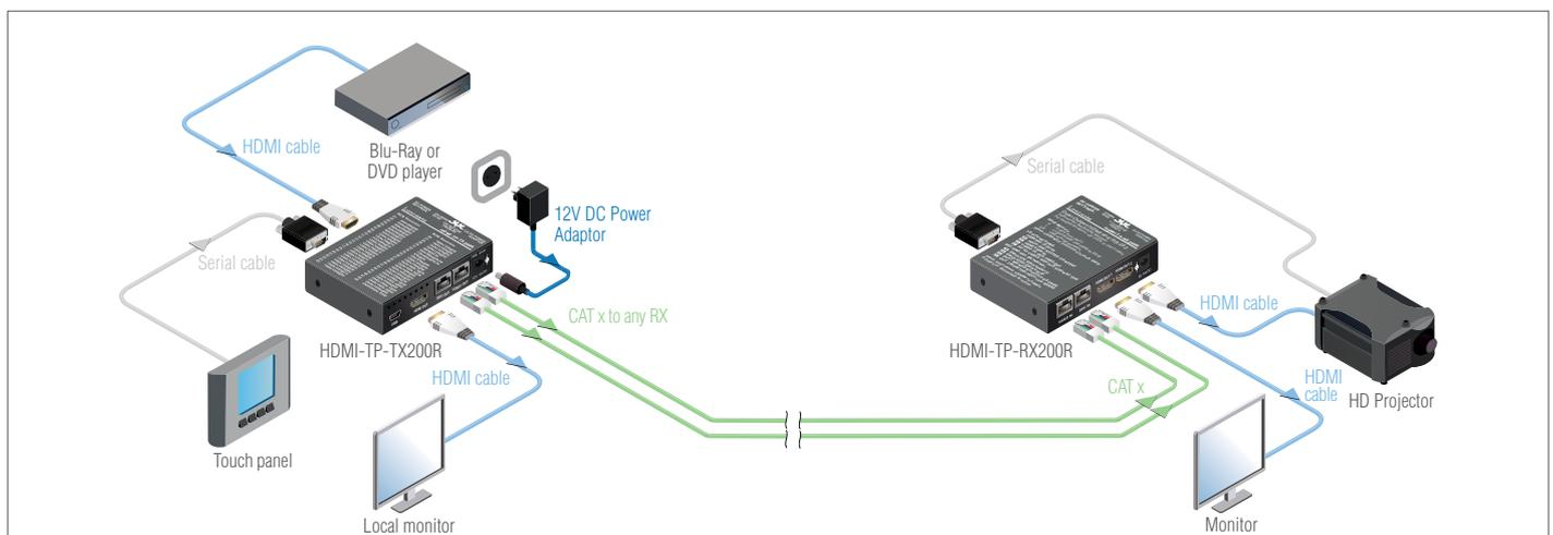
**Dual Output** is available on both units through a built-in distribution amplifier. HDMI-TP-TX200R has a local monitor HDMI output to enable easy monitoring of the outgoing signal and HDMI-TP-RX200R has two identical HDMI Outputs.
