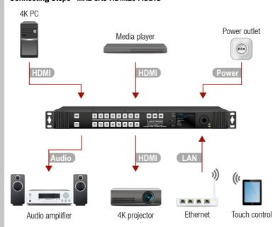
HDMI Connect the desired source to an HDMI input port.
